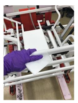
4.15 Using the bed lifter, begin to tilt the bed frame, to access areas underneath. Please note, do not alter the set max tilt angle of the forks. You should also ensure that the handle is moved out of the way (to the side position) when beds are worked on, which will prevent damage to the handle.
